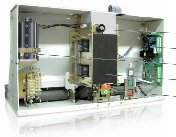
Emergency manual breaking mechanism
